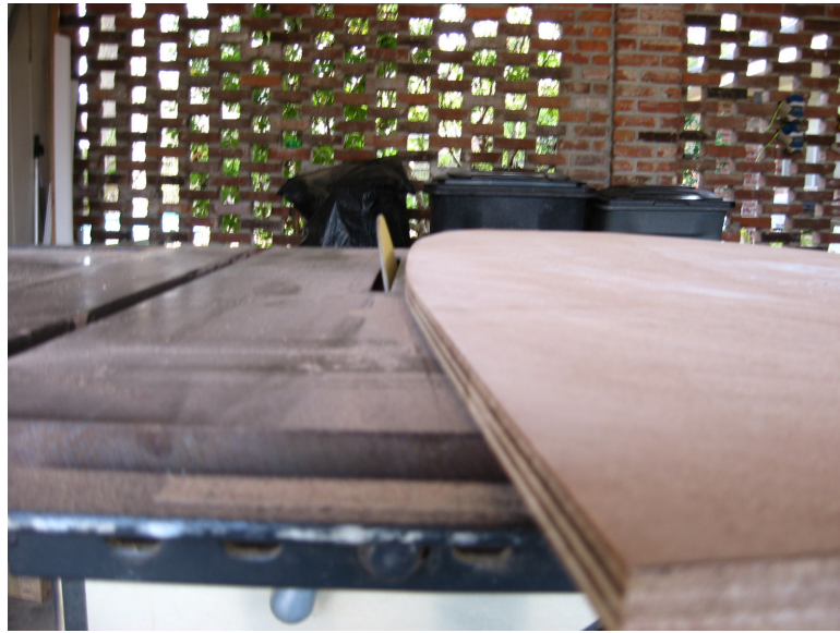
Figure 25 Table saw sanding disc set to make angle for hull abutment
