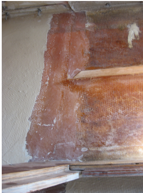
Figure 6 Tabbing on shelf left intact but cut back from bulkhead
