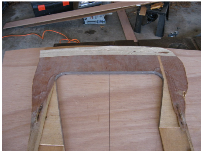
Figure 7 Old bulkhead used as pattern for anchor locker access
