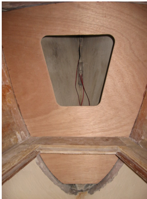
Figure 12 Bulkhead dry fitted
