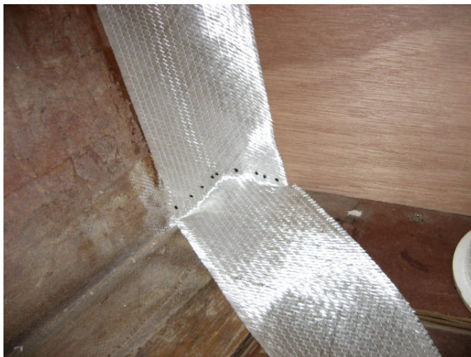
Figure 17 Tabbing tape marked for cutting
