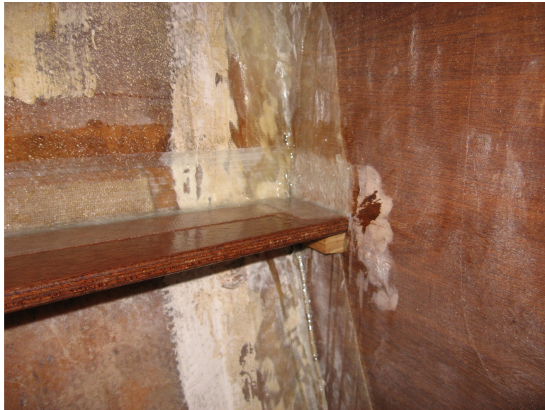
Figure 29 Shelf cleats and end tabbing
