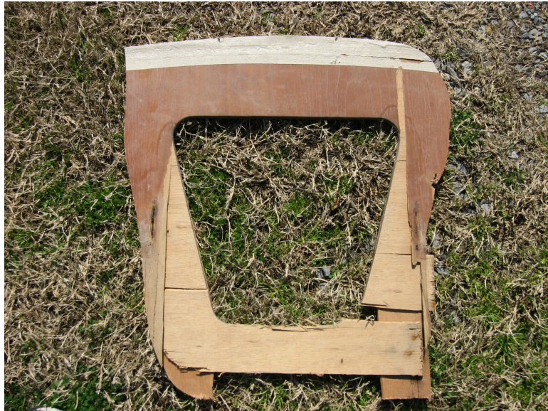
Figure 2 Center of old bulkhead cut out for pattern for anchor locker access
