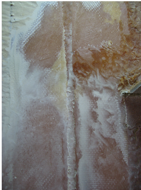
Figure 4 All tabbing removed and surface smoothed
