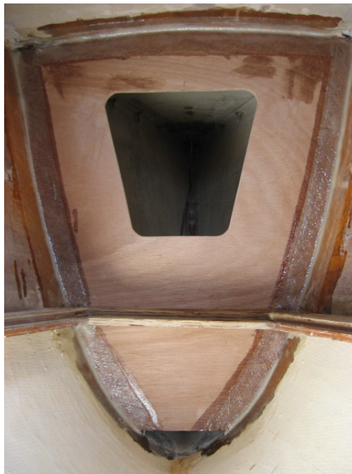
Figure 21 Bulkhead installed and tabbed
