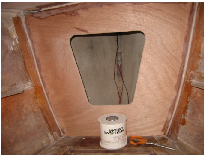
Figure 16 Fillet finished. Ready to apply tabbing
