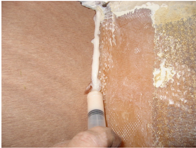
Figure 14 Thickened epoxy being applied for fillet
