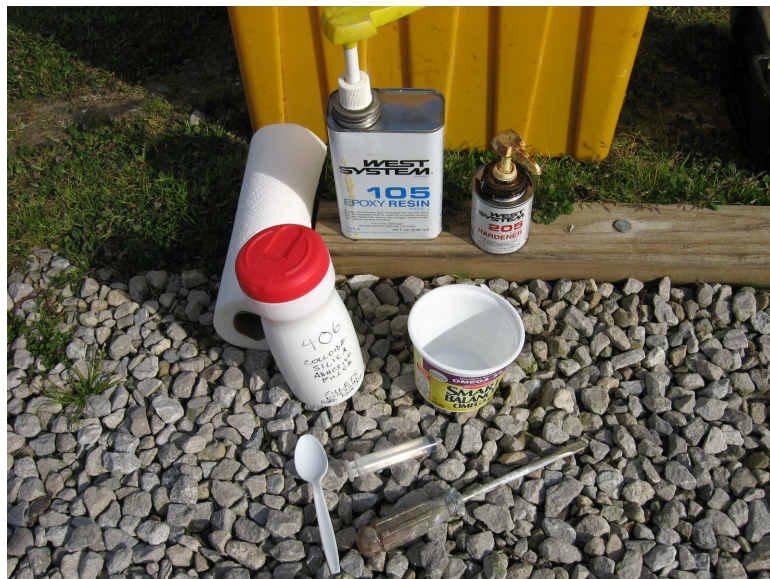
Figure 13 Materials needed for filleting
