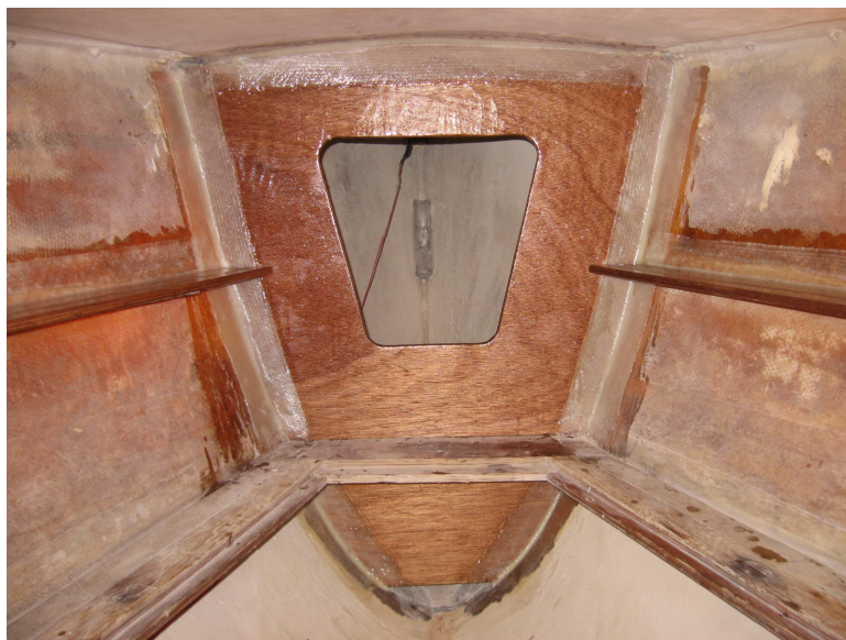
Figure 28 Installed shelf (minus cleats)
