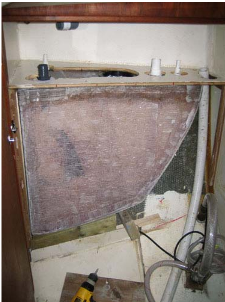
Tank in head – strong frame underneath and a tube of 4200 between hull and tank
