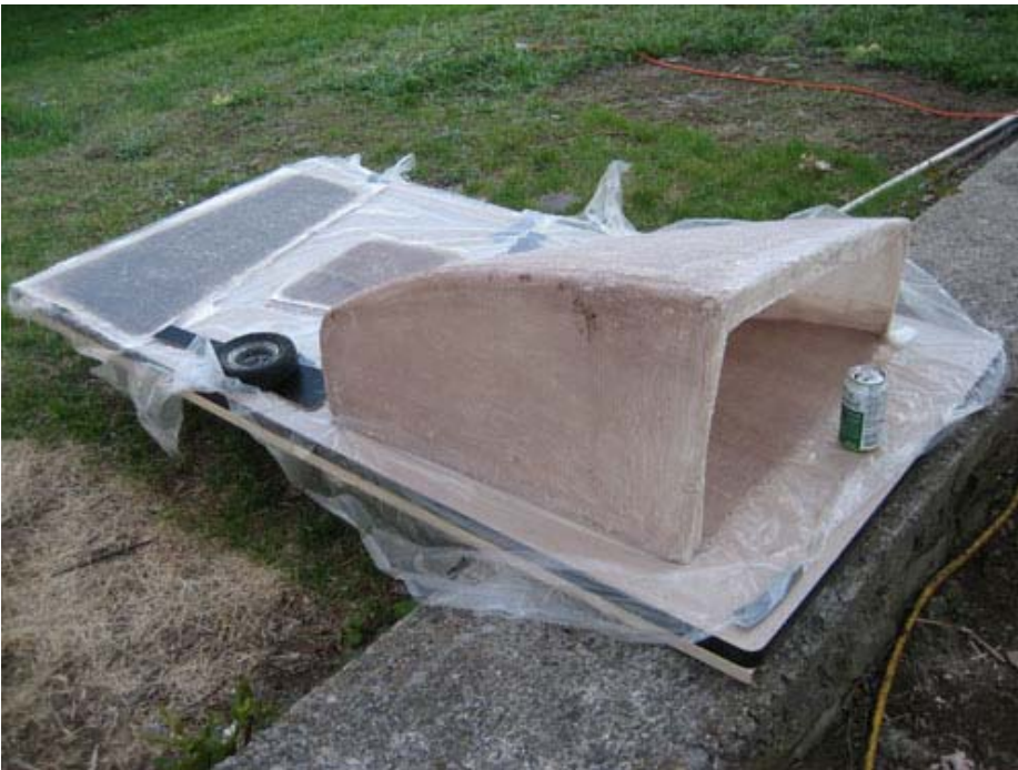
Finish the inside's top tab (not shown) with the help of a steel L bar to hold the vertical shape to receive the top.
