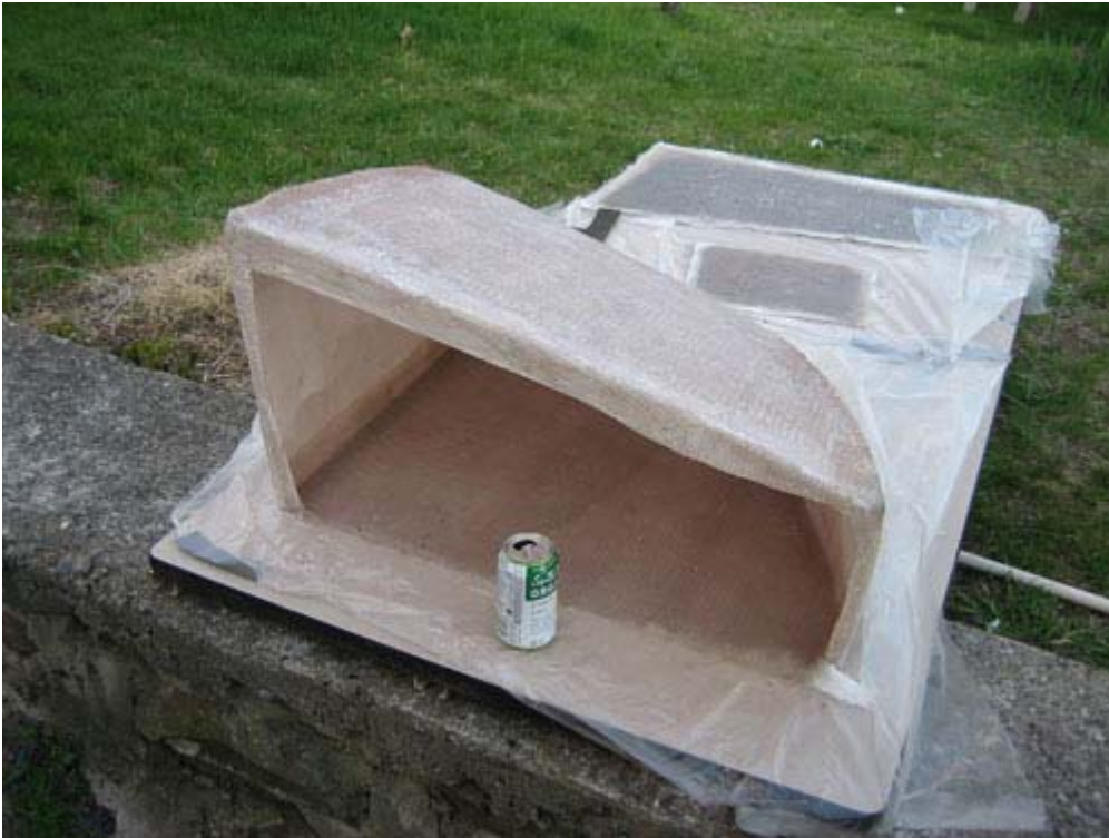
Finished tank without lid and baffle installed (in background)
